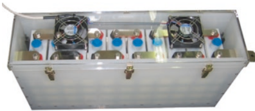
Abb. 7.41 Nickel-Metall-Hydrid-Modul Hoppecke 75 Ah/ 10 Zellen
